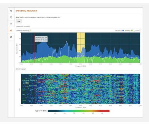
The spectrum analyzer tool has been improved by adding a waterfall chart. The screenshot above shows a very high interference, which also complicates the communication of the link.
